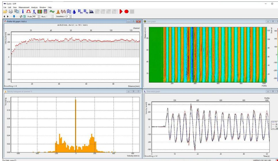
Velocity profile measurement of a piston cyclic flow
