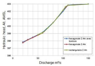
Figure 11: Rating curves for three different orifice geometries, proving the appropriate choice of the hexagonal one.
