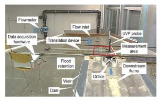
Figure 2: Partial view of the Aire River physical model at the LHA of HEPIA, with the flow monitoring facilities installed upstream from the discharge limiting orifice.
