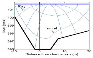
Figure 12: Orthogonal Ray-Isovel network taken into account for shear stress analysis in the upstream vicinity of the orifice.
