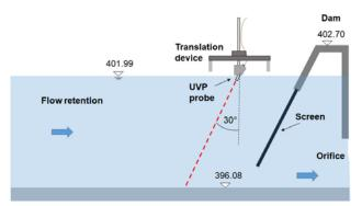
Figure 4: UVP probe implemented upstream from the discharge limiting orifice of the dam.
