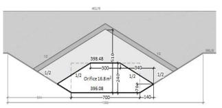
Figure 10: Discharge limiting orifice, with a 9.8 m large, 2.4 m high hexagonal bottom opening of the dam.
