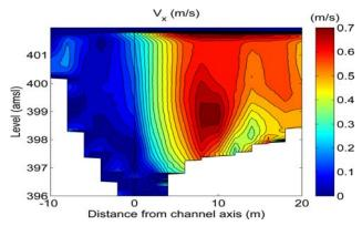
Figure 9: Flow map achieved on the physical model. Velocity vector field, Vx, perpendicular to the channel axis. Core velocity found close to rack of the gravel pit.
