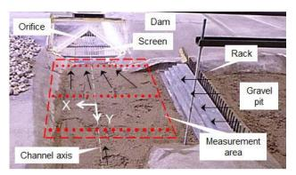
Figure 3: Upstream view of the dam showing the UVP measurement scheme composed of 16 points set in 3 rows.
