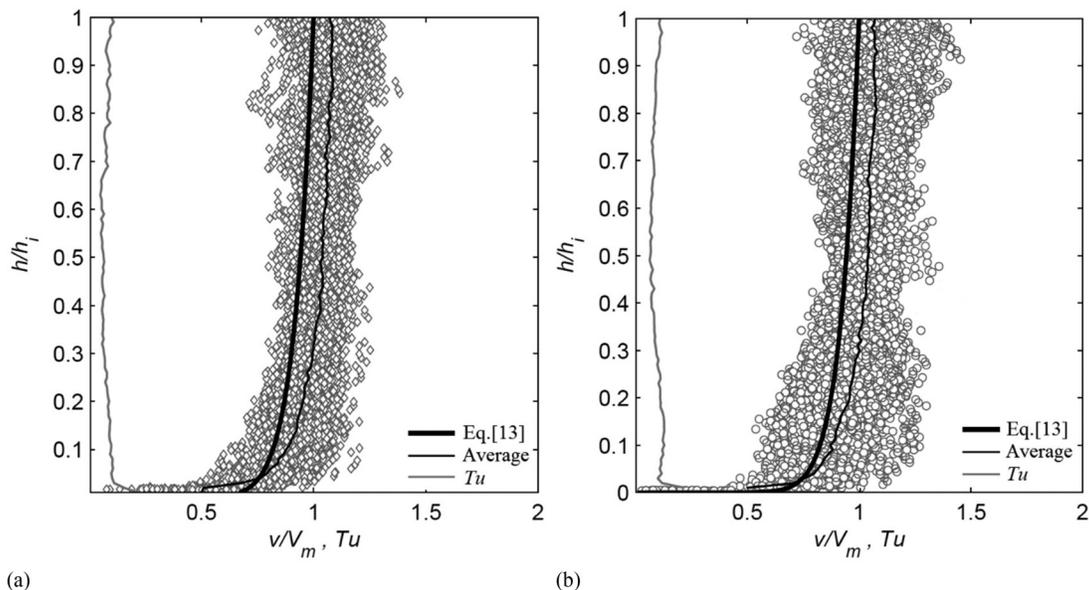
**Fig. 19.** Normalized velocity profiles and turbulent intensity,  $Tu$ , for  $T \cdot (g/d_0)^{0.5} < 42$ : (a) dry bed surge (160 profiles Test 1); (b) wet bed bore with  $d_0 = 0.82$  m and  $h_0 = 0.05$  m (104 profiles, Test 11)
