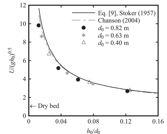
**Fig. 17.** Average bore front celerity,  $U$ , as a function of the initial still water depth,  $h_0$ ; experimental results compared to the momentum equation [Eq. (9)] and the numerical approximation proposed by Chanson (2004), shown in Eq. (10), for different impoundment depths:  $d_0$  was 0.82 m for Tests 4, 5, 8, 11, and 14;  $d_0$  was 0.63 m for Tests 6, 9, and 12; and  $d_0$  was 0.40 m for Tests 7, 10, and 13
