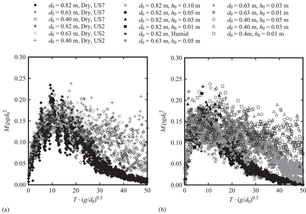
**Fig. 23.** Momentum,  $M = \rho \cdot h \cdot V_m^2$ , computed for (a) dry bed surges and (b) wet bed bores for various impoundment depths, denoted  $d_0$ , and initial still water depths, denoted  $h_0$
