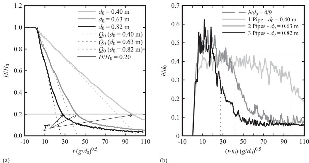
**Fig. 5.** Measurements of the water depth for three dry bed surges generated with the vertical release technique using one, two, and three pipes in Tests 3, 2, and 1, respectively: (a) upstream reservoir; (b) channel inlet ( $x = 0$  m) (Note: the values of the released discharges are presented in Table 1)
