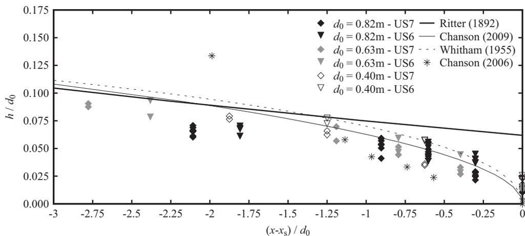
**Fig. 10.** Comparison of the measured longitudinal wave profiles with the theoretical solutions of Ritter (1892), Whitham (1955), Chanson (2009), and prototype data (Chanson 2006) in the wave-tip region where  $x$  was  $13.85$  and  $13.60$  m for US7 and US6, respectively
