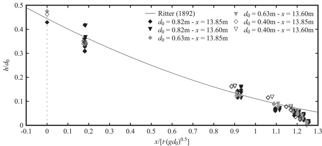
**Fig. 9.** Longitudinal dimensionless water surface profiles when the wave reached two measurement locations, at  $x = 13.60$  and  $13.85$  m for US6 and US7, respectively; comparison of all generated surges with  $d_0$  values of  $0.82$ ,  $0.63$ , and  $0.40$  m with the theoretical solutions from Ritter (1892)
