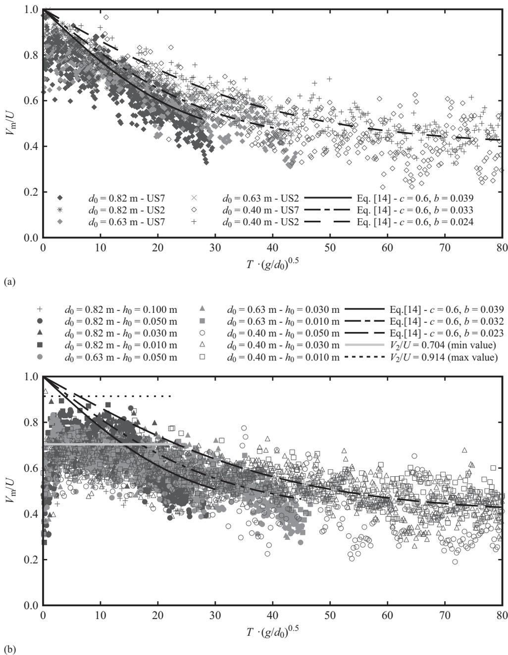
**Fig. 20.** (a) Dimensionless depth-averaged velocities,  $V_m/U$ , for 12 dry bed surges with different impoundment depths at two different locations at  $x$  of 13.85 and 10.20 m for US7 and US2, respectively; (b) dimensionless depth-averaged velocities,  $V_m/U$ , for 19 wet bed bores with different impoundment depths and initial still water depths at a fixed location,  $x = 13.85$  m
