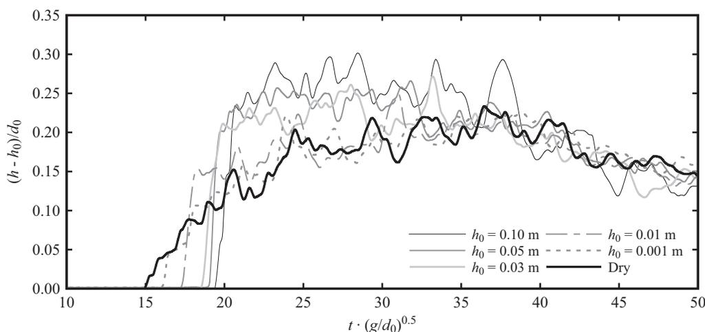
**Fig. 12.** Bore profiles for waves with different initial still water depths at  $x$  of 13.85 m (US7) for  $d_0$  of 0.82 m with all profiles brought down to  $(h-h_0)/d_0$  for Tests 1, 4, 5, 8, 11, and 14
