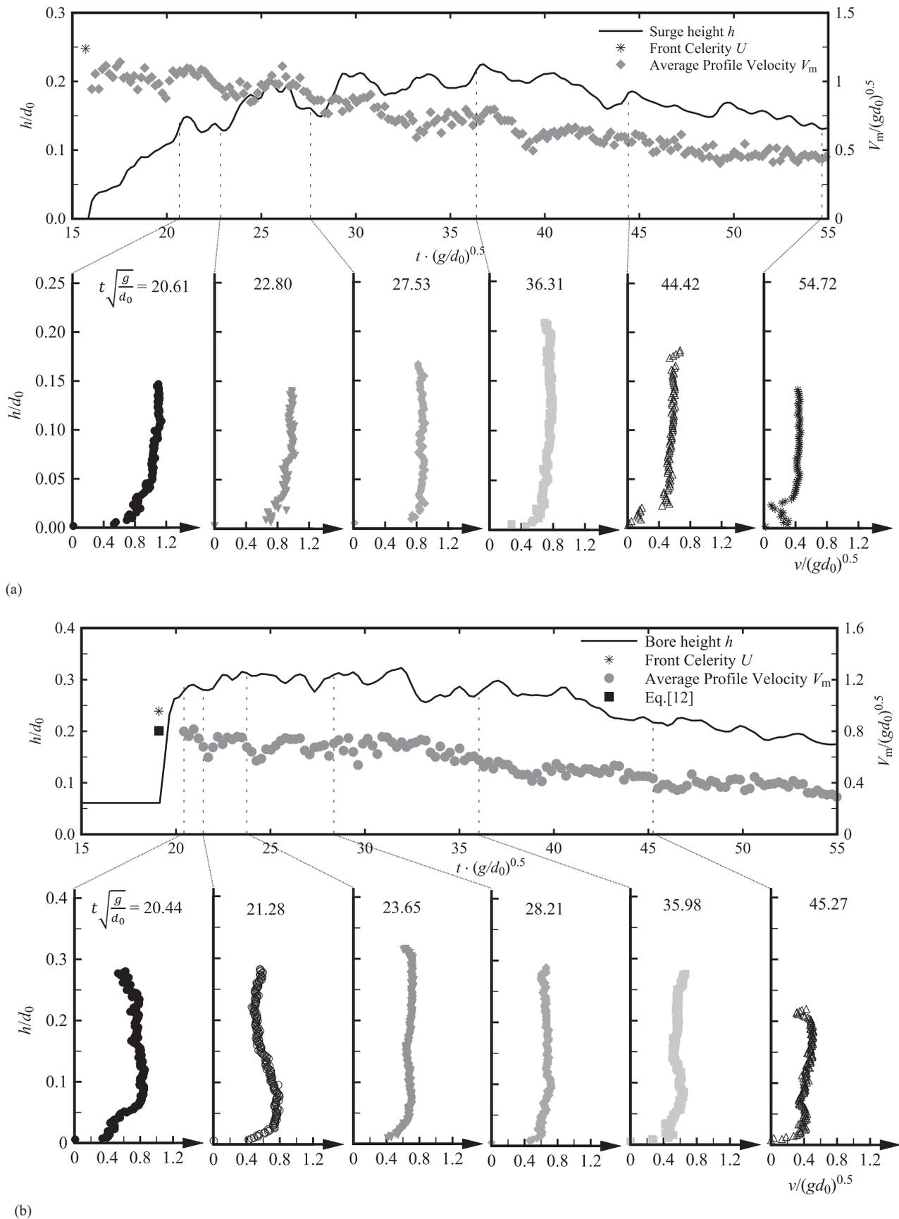
**Fig. 18.** Wave height,  $h$ , depth-averaged velocity,  $V_m$ , and velocity profiles at specific times for (a) dry bed surge with  $d_0 = 0.82$  m for Test 1 and (b) wet bed bore with  $d_0 = 0.82$  m and  $h_0 = 0.050$  m for Test 11, both measured at  $x$  of 13.85 m (US7) from the channel inlet
