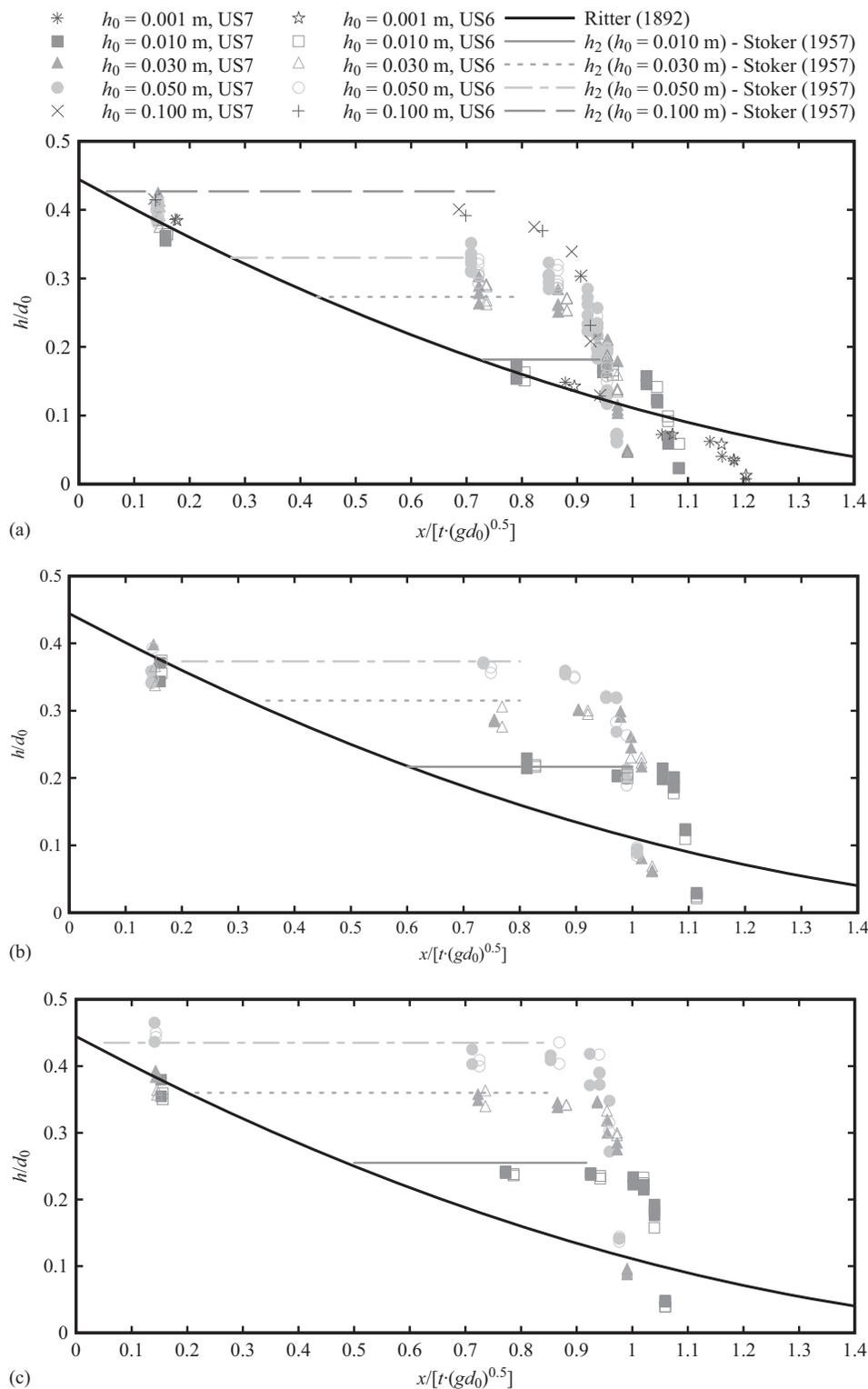
**Fig. 13.** Longitudinal free-surface profile for bores with different initial still water depths, denoted  $h_0$ , and impoundment depths, denoted  $d_0$ , compared with the theoretical solutions of Ritter (1892) and the plateau heights, denoted  $h_2$ , obtained with Eq. (5) (Chanson et al. 2000); measurements at US 7 (solid symbols) and US 6 (empty symbols): (a)  $d_0 = 0.82$  m; (b)  $d_0 = 0.63$  m; (c)  $d_0 = 0.40$  m
