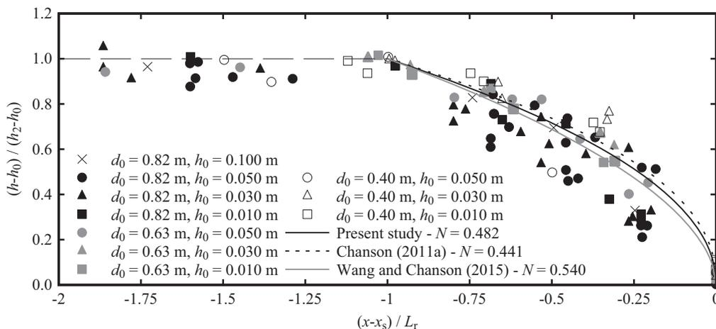
**Fig. 15.** Normalized bore front profiles, for various values of  $d_0$  and  $h_0$ , for comparisons of the experimental data from the proposed vertical release technique with data from the empirical formulas from Chanson (2011) [Eq. (6)] and from Wang and Chanson (2015) for hydraulic jumps
