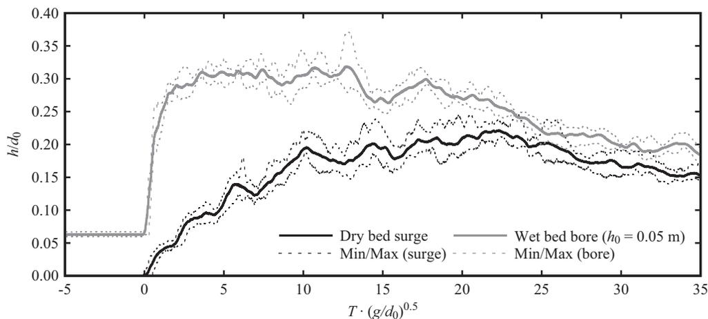
**Fig. 6.** Repeatability for dry bed surges (three pipes,  $d_0 = 0.82$  m, Test 1, eight repetitions) and wet bed bores with three pipes, (three pipes,  $d_0 = 0.82$  m,  $h_0 = 0.05$  m, Test 11, five repetitions) measured at  $x$  of 13.85 m (US7)
