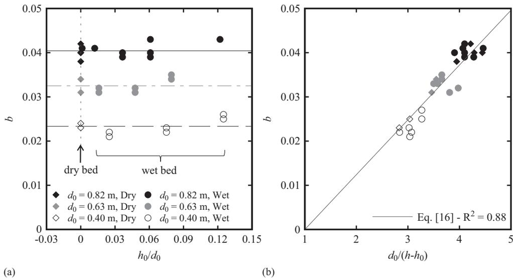
**Fig. 21.** Definition of parameter  $b$  in Eq. (15): (a) Eq. (15a) function of  $h_0/d_0$ ; (b) Eq. (15b) function of  $d_0/(h-h_0)$ , where  $h$  equals  $h_{\max}$  for surges and  $h$  equals  $h_2$  for bores (Note: Same legend applies to both panels)
