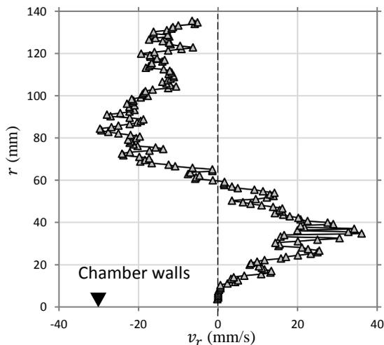
Figure 6: Radial velocity profile at transducers T8
