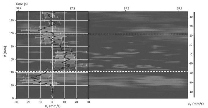
Figure 8: Axial velocity profile at transducers T4
