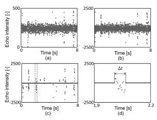
Figure 4: Time traces of echo intensity; (a) raw data, (b) processing Laplacian filter, (c) elimination of small intensities by thresholding, and (d) enlarged view at a part of strong echo intensity scattered by a larger particle
