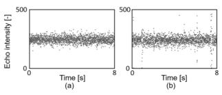
Figure 3: Time traces of echo intensity for (a) only smaller particles, and (b) smaller and larger particles
