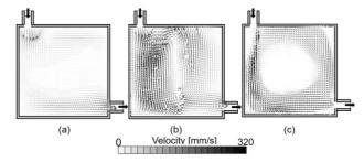
Figure 7: Comparison of velocity vector distributions estimated from (a) velocity data measured by Doppler velocimetry, (b) velocity data measured by Doppler velocimetry and echo intensity method, and (c) corresponding velocity field measured by PIV
