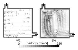
Figure 6: Velocity vectors distribution obtained from (a) Doppler velocimetry and echo intensity method, and (b) after processing LER and VCP
