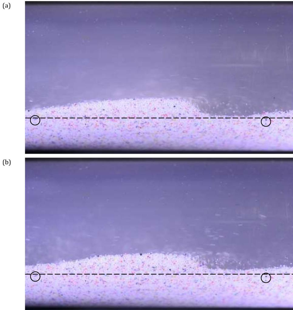
**Fig. 13.** Images of flow over regular ripple bed ( $Q=0.191 \text{ l s}^{-1}$ ,  $\phi_w=0.5\%$ ; 1920 by 1080 pixels, 75.7 by 42.6 mm). Dashed lines represent boundary between stationary and moving parts of bed, from inspection of detail in images. Images (a) and (b) from same run, separated in time by  $\Delta t \approx 3.5$  minutes and showing different ripples. Circled areas show examples of common bed features in stationary part of bed.
