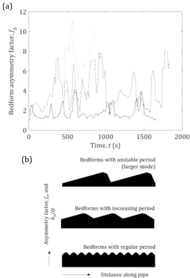
**Fig. 12.** (a) Bedform asymmetry factor,  $f_b$ , against time for regular ripples (solid black line;  $Q=0.498$  to  $0.402$   $\text{l s}^{-1}$  at  $t=0$ ,  $\phi_w=0.1\%$ ), ripples with increasing period (dashed black line;  $Q=0.483$  to  $0.323$   $\text{l s}^{-1}$  at  $t=0$ ,  $\phi_w=0.5\%$ ) and unstable/cyclic bedforms (solid gray line;  $Q=0.383$  to  $0.287$   $\text{l s}^{-1}$  at  $t=0$ ,  $\phi_w=1\%$ ); (b) schematic summary of bedform types.
