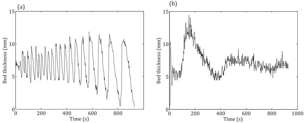
**Fig. 6.** Bed thickness against time from acoustic data, showing hysteresis behavior, (a)  $Q=0.483$  to  $0.323$  l  $s^{-1}$  at  $t=0$ , (b)  $Q=0.323$  to  $0.483$  l  $s^{-1}$  at  $t=0$  ( $|\Delta Q|=0.160$  l  $s^{-1}$ ,  $\phi_w=0.5\%$ ). Runs were performed concurrently.
