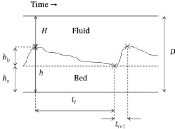
**Fig. 1.** Time-dependent bedform geometry and evolution.  $H$  and  $h$  are fluid and bed depths, with  $h = h_b + h_s$ , where  $h_b$  and  $h_s$  are bedform height and settled bed depth, respectively.  $R$  and  $D$  are pipe radius and diameter;  $t_i$  is  $i^{\text{th}}$  period between adjacent peak and trough.
