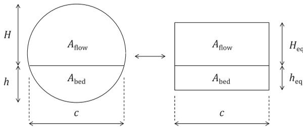
**Fig. 15.** Illustration of a suggested universal scaling for closed-conduit flows of any cross-sectional shape.
