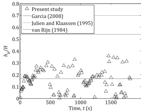
**Fig. 11.** Scaling and evolution of bedform height,  $h_b$ , relative fluid height,  $H$ , against time,  $t$ , for case of unstable/cyclic bedform field alternating between ripples and dunes ( $Q=0.383$  to  $0.287$   $l\ s^{-1}$  at  $t=0$ ,  $\phi_w=1\%$ ).
