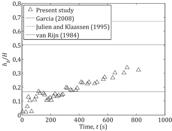
**Fig. 10.** Scaling and evolution of bedform height,  $h_b$ , relative to fluid height,  $H$ , against time,  $t$ , for case of bedform field of increasing period ( $Q=0.483$  to  $0.323$   $l\ s^{-1}$  at  $t=0$ ,  $\phi_w=0.5\%$ ).
