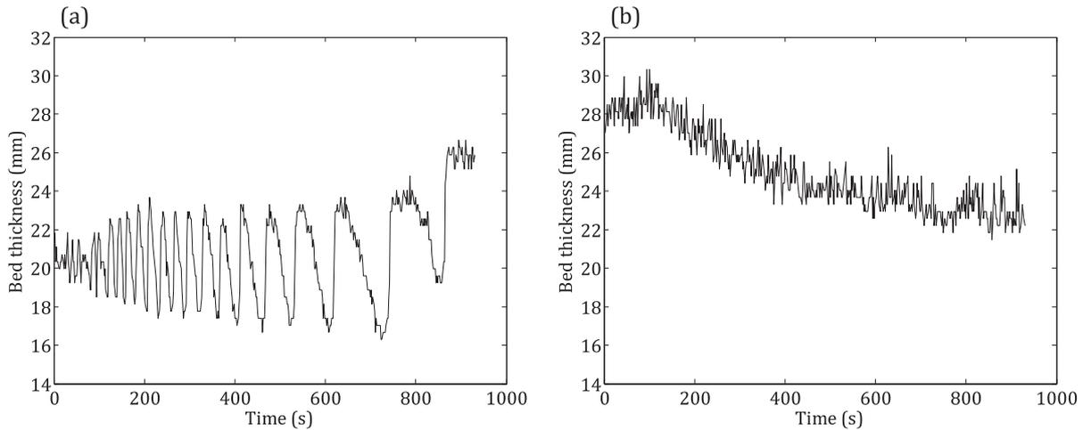
**Fig. 7.** Bed thickness against time from acoustic data, showing hysteresis behavior, (a)  $Q=0.342$  to  $0.277$  l  $s^{-1}$  at  $t=0$ , (b)  $Q=0.277$  to  $0.342$  l  $s^{-1}$  at  $t=0$  ( $|\Delta Q|=0.065$  l  $s^{-1}$ ,  $\phi_w=3\%$ ). Runs were *not* performed concurrently.
