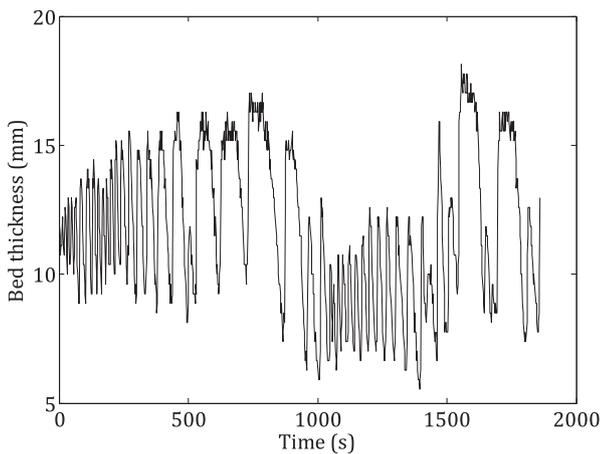
**Fig. 4.** Bed thickness against time: unstable and cyclic ripple-to-dune formation ( $Q=0.383$  to  $0.287$  l s<sup>-1</sup> at  $t=0$ ,  $\phi_w=1\%$ ).
