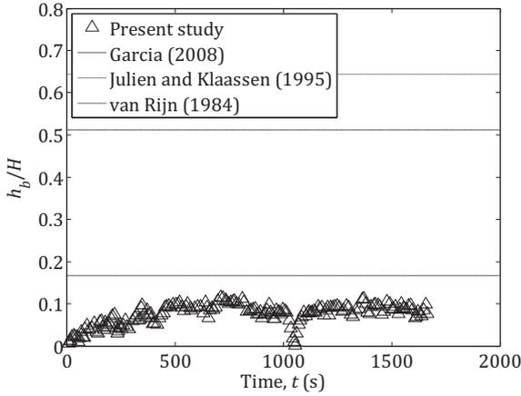
**Fig. 9.** Scaling and evolution of bedform height,  $h_b$ , relative to fluid height,  $H$ , against time,  $t$ , for case of ripple bedform field of regular period ( $Q=0.498$  to  $0.402$   $l\ s^{-1}$  at  $t=0$ ,  $\phi_w=0.1\%$ ).
