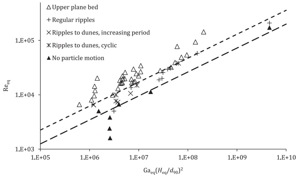
**Fig. 16.** Phase diagram of bedforms in pipe flow according to equivalent Reynolds number,  $Re_{eq}$  against  $Ga_{eq}(H_{eq}/d_{90})^2$ . Unfilled triangles: upper plane bed; pluses: regular ripples; crosses: unstable ripple-to-dune cycles; stars: ripples that transition with increasing period to dunes; filled triangles: no particle motion. Dashed lines indicate transitions between no particle motion, time-dependent bedform fields and upper plane beds, and are visually fitted.
