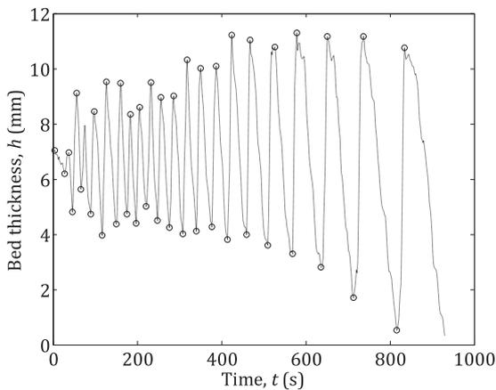
**Fig. 8.** Total bed thickness,  $h$ , against time for case of bedform field of increasing period, with ripple-to-dune transition ( $Q=0.483$  to  $0.323$  l  $s^{-1}$  at  $t=0$ ,  $\phi_w=0.5\%$ ). Circles indicate local minima and maxima (*i.e.* peaks and troughs).
