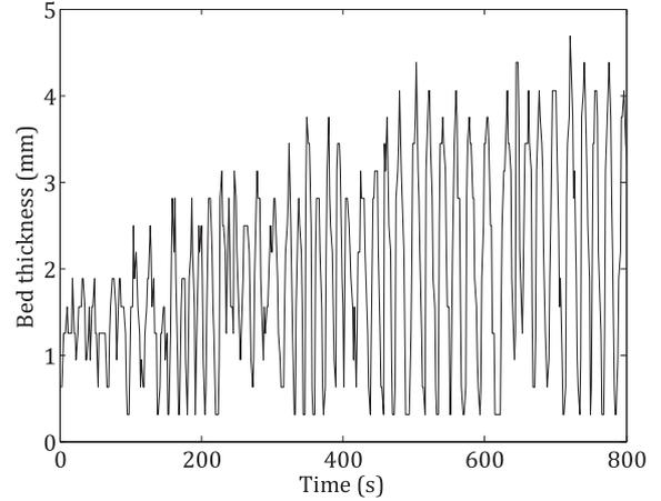
**Fig. 2.** Bed thickness against time: shallow, regular ripples ( $Q=0.498$  to  $0.403 \text{ l s}^{-1}$  at  $t=0$ ,  $\phi_w=0.1\%$ ).
