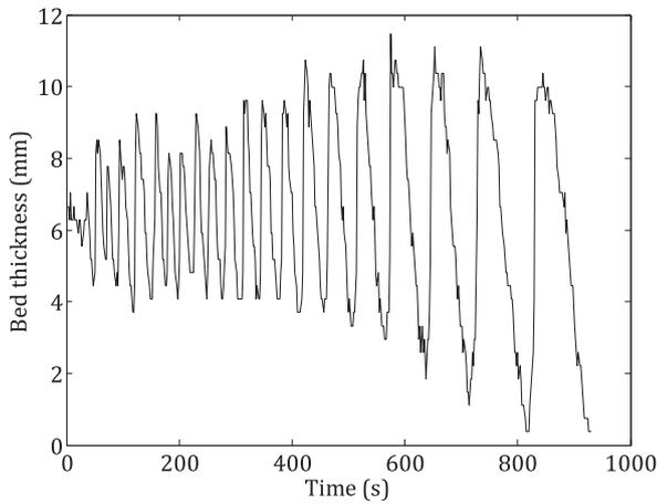
**Fig. 3.** Bed thickness against time: transitioning ripple-to-dune formation with increasing period ( $Q=0.483$  to  $0.323$  l s<sup>-1</sup> at  $t=0$ ,  $\phi_w=0.5\%$ ).
