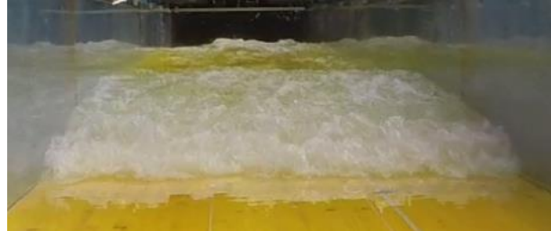
Figure 4 : Picture of the wet bed bore ( h_0 = 0.05 m)
