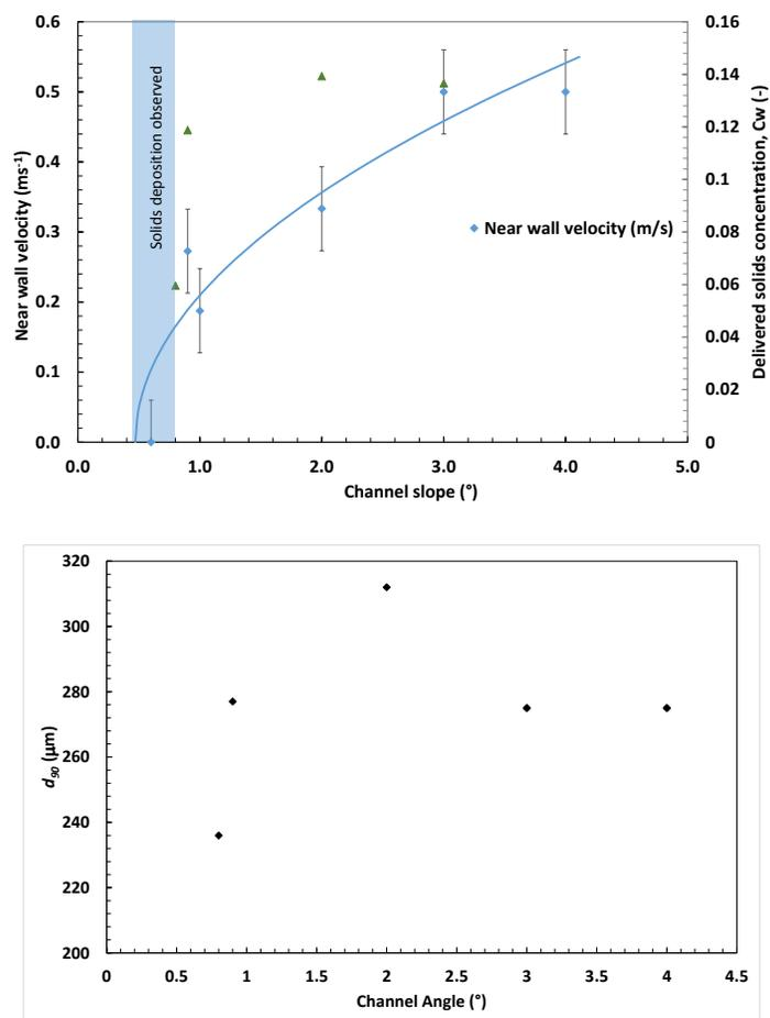
**Figure 7** (above) Near wall velocity in open channel measured by deposition probe for constant flow rate (140 L/min). Delivered solids concentration are shown on the right hand axis. (below)  $d_{90}$  of delivered solids
