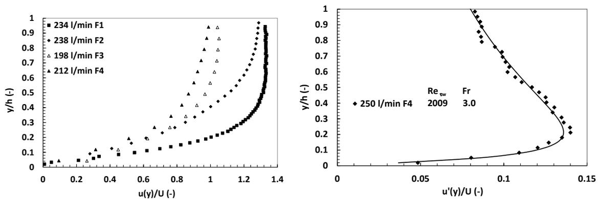
Figure 5 UDVP centerline axial velocities for particle free runs 2° slope. Velocities with depth,  $u(y)$ , are normalized over mean axial velocity  $U$ . Distance above invert,  $y$ , is normalized over depth,  $h$
