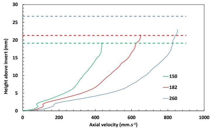
**Figure 6** Velocity profile measured by UDVP for channel centerline (F4 fluid, 2° slope) free surface shown by broken line. Legend in L.min-1
