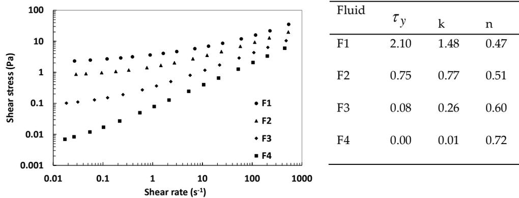
Figure 4 (left) Rheogram of Carbopol solutions used as carrier fluid in channel trials. (right) Herschel Bulkley model parameters for test fluids
