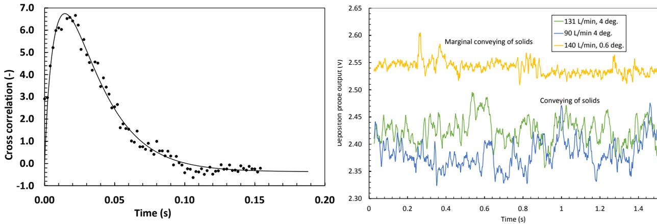
**Figure 3** (left) Deposition probe output at varying flow conditions. (right) Sample cross correlation output.
