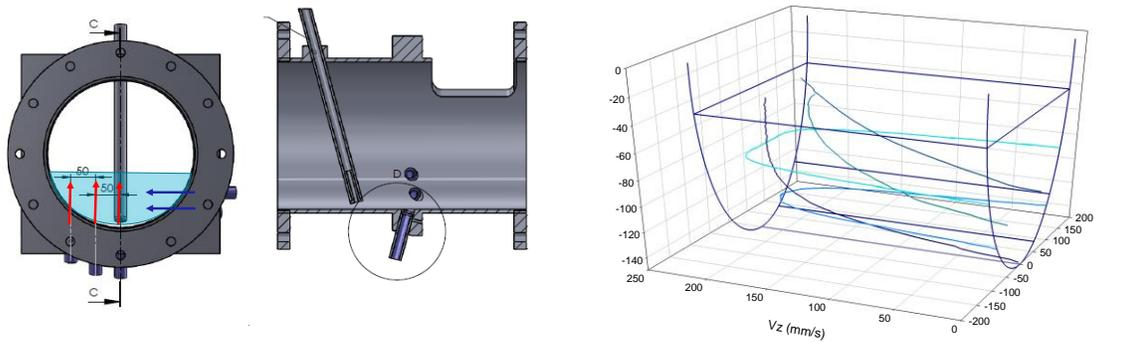
**Figure 2** (left) Sectioned view of the UDVP probe module. Arrows indicate location of measured velocity profile. (right) UDVP velocity profiles from 5 transducers (F1, 247 L.min-1, slope 0.5°)
