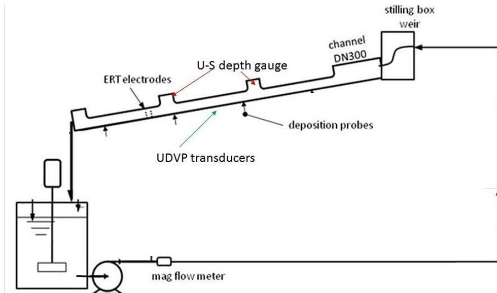
**Figure 1** Schematic of the 300 mm diameter, 20 m long inclinable flume test facility
