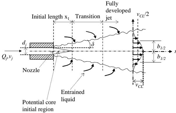
Figure 3: Jet flow behavior according to [7].
