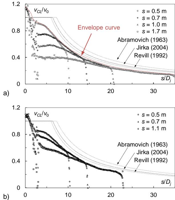
Figure 4: Dimensionless jet centerline velocity  $v_{CL}/v_0$  as a function of dimensionless distance  $s/D_j$  from the nozzle. Comparison between experiments and values from literature. 0.5 MHz UVP sampling for  $Q_{IN} = 0.7$  l/s (a) and 1.0 MHz UVP sampling for  $Q_{IN} = 0.5$  l/s (b).
