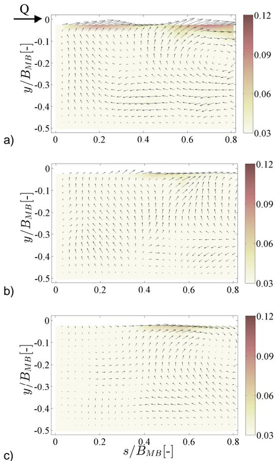
Figure 5: Sampled flow patterns for a jet entering at  $s/B_{MB} = y/B_{MB} = 0$  and  $z/B_{MB} = 0.25$ , for  $Kt_P = 0.8$  and  $Q = 0.7$  (a & b) and  $1.1$  l/s (c). Dimensionless velocity  $v/v_0$  at  $z/B_{MB} = 0.25$  (a, at jet axis) and  $0.125$  (b & c, below jet axis).
