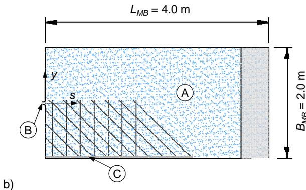
Figure 1: Picture of test facility (a) and schematic plan view of the main basin (b). A is the main basin; B, the intake/outlet; C, the UVP-frame with indicated 2D velocity sampling grid, and D, the mixing tank.
