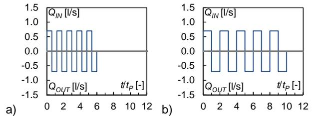
Figure 2: Configurations of tested in- and outflow cycles, example for  $Q = 0.7$  l/s and  $Kt_p = 0.6$  (a) and  $1.0$  (b).
