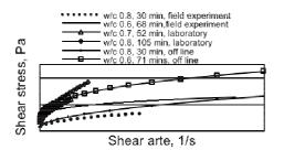
Figure 5 Shear stress vs. shear rate curve for different w/c ratio
