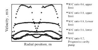
Figure 3 Velocity profiles measured by UVP
