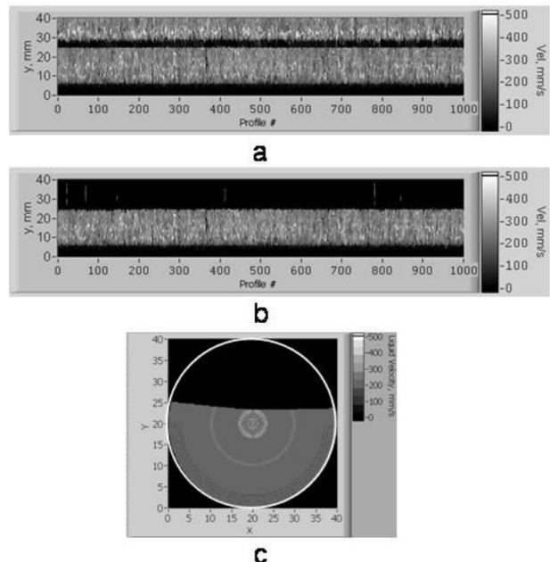
Figure 6.  $Q_a=0.6$ ;  $\alpha=10\%$  a) Raw data b) Processed data c) liquid phase velocity distribution, profile #50
