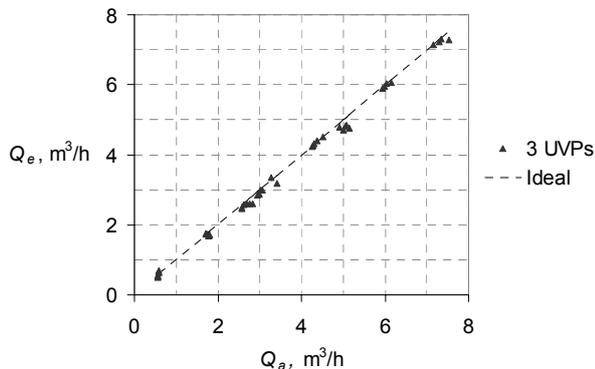
Figure 4. Estimated liquid flow rate,  $Q_e$  versus actual liquid flow rate,  $Q_a$
