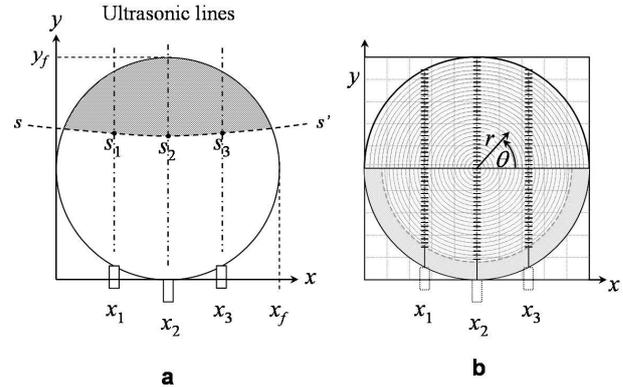
Figure 3. a) Gas-liquid interface height position b) Channel distribution
