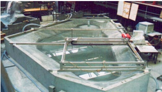
Figure 5: The physical scale model of the Essert compensation basin, UVP probes fixed on a 3D traversing frame
