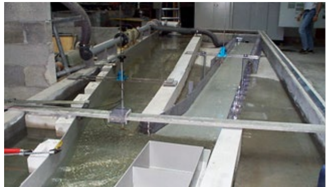
Figure 7: Physical model of the waste loading station facility at the junction of the Rhone and Arve Rivers in Geneva
