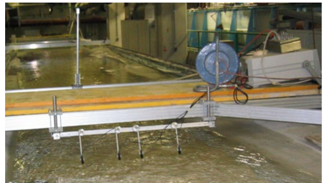
Figure 8: UVP transducers mounted on the measurement platform over the gravel pit in the physical model
