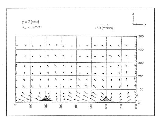
Fig. 3: Horizontal flow mapping of one plane
