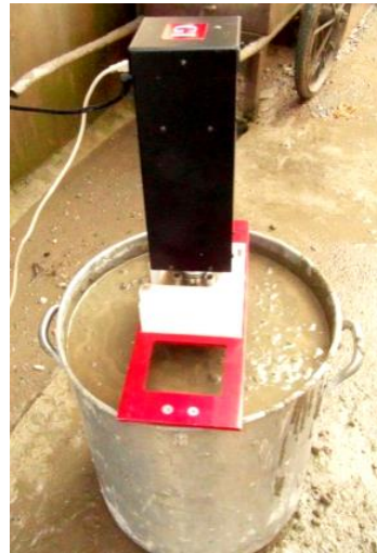
Figure 4. Measuring the rheological parameters of fresh concrete using the ICAR rheometer.
