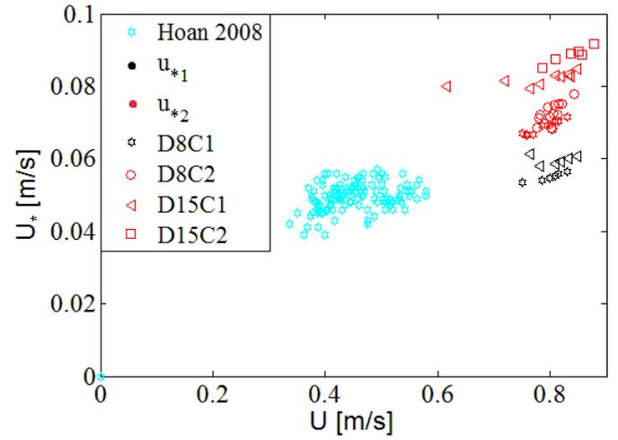
Figure 5. Computed shear velocity with eq. 2 and eq. 3
