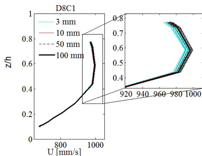
Figure 2. Velocity profile over a rough bed, ( $d=8$  mm), for a discharge of 15 l/s. Averages over 3 mm, 10 mm, 50 mm and 100 mm along the main flow direction.
