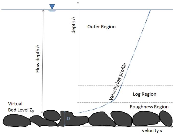
Figure 6. Layers of an open channel flow over a rough bed
