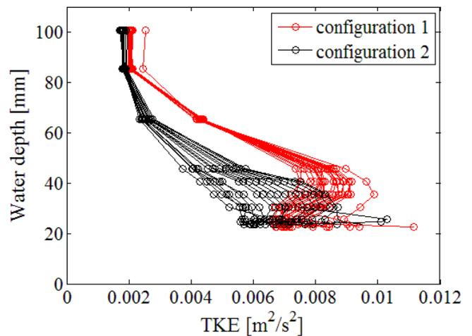
Figure 8. TKE profile along X-axis in a flow of  $Q=16$  l/s, over sediments of 15 mm diameter)
