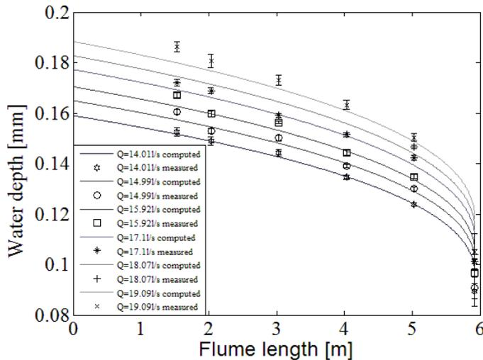
Figure 4 Comparison between computed water surface profile and the measured values, with roughness factor of  $k_s$  (wall) = 0.00002 m and  $k_s$  (bottom) = 0.015 m
