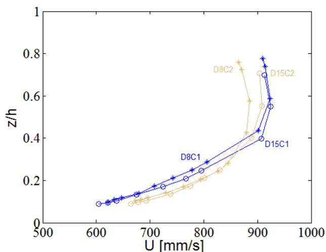
Figure 3. Velocity profile over a rough bed, respectively over a smooth-to-rough transition, ( $d=8$  mm and  $d=15$  mm), for a discharge of 15 l/s.
