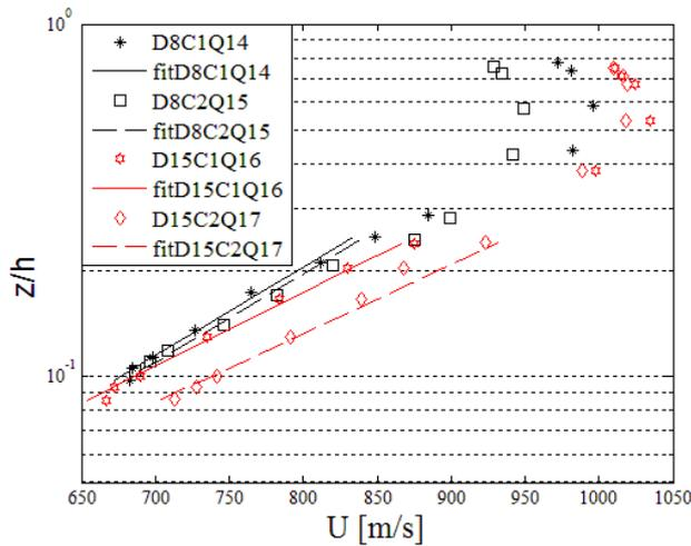
Figure 7. Fit of eq. 3 with the measurements for diameter 8 mm (D8), respectively 15 mm (D15), both configuration (C1 and C2), discharge between 14 l/s and 17 l/s
