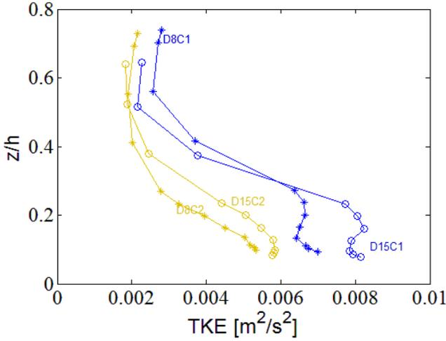
Figure 9. TKE profiles over a rough bed, respectively transition smooth-to-rough, ( $d=8$  mm and  $d=15$  mm), for a discharge of 16 l/s.
