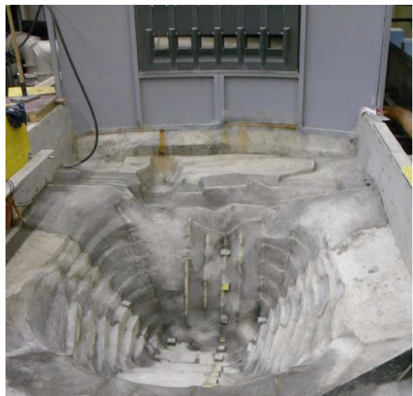
Figure 1. Physical model at LCH, view from upstream of Kariba dam orifice spillways with two stop-logs (top), view from downstream of the plunge pool towards the dam (bottom).
