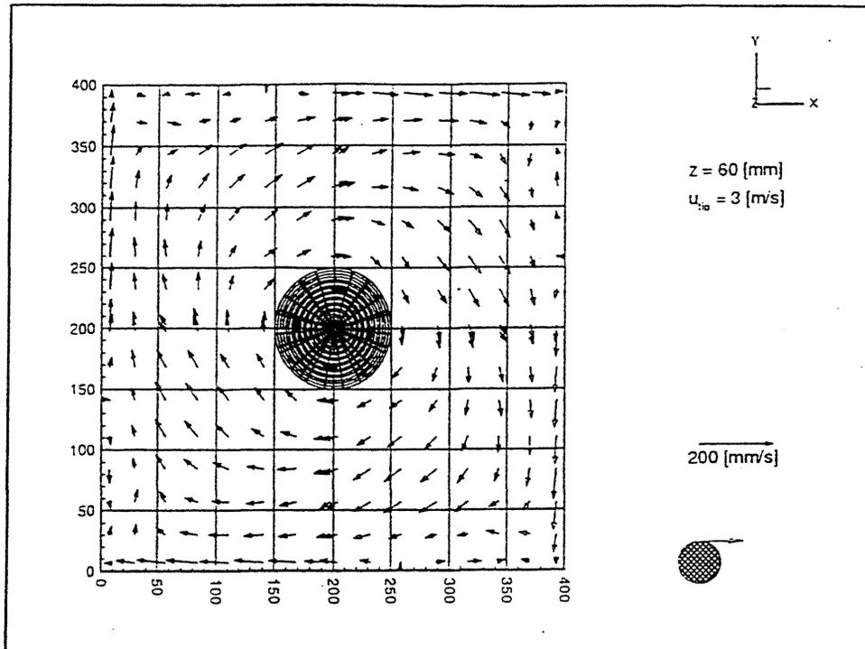
Fig. 4: Vertical flow mapping of one plane
