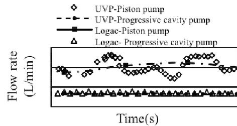
Figure 4 Comparison of the volumetric flow rate determined by the UVP and measured by the LOGAC
