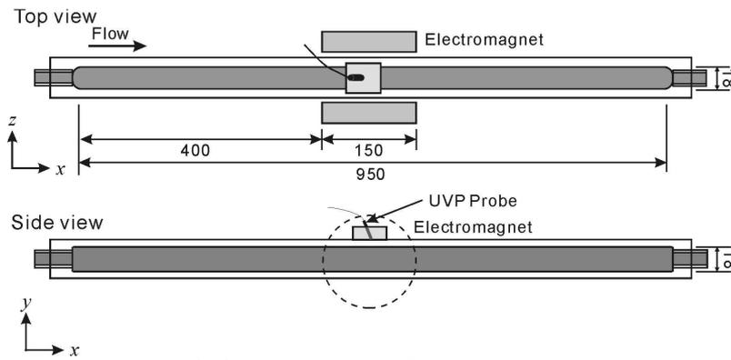
Figure 1: Detailed structure of the rectangular duct.
