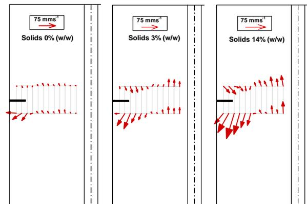
Figure 5 Time-averaged 2D velocity vectors for *low flow*
