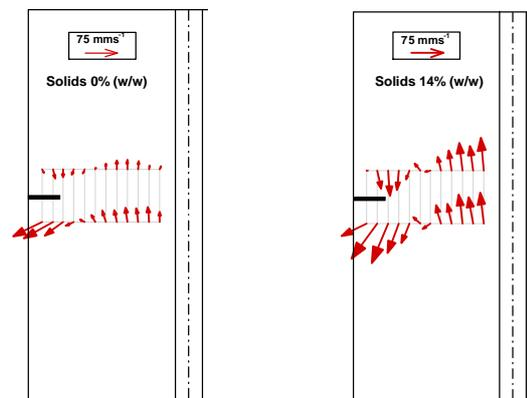
Figure 6 Averaged 2D velocity vectors for *high flow*
