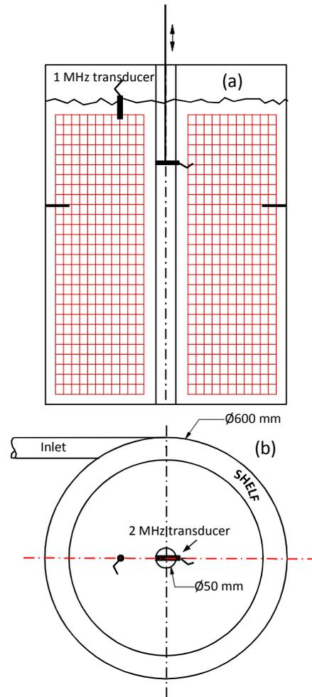
Figure 2 Measurement schematic
