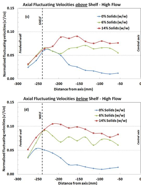
Figure 7 Axial fluctuating velocities above and below the feedwell shelf measured by UVP high flow
