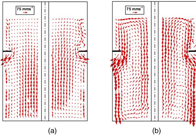
Figure 3 Detailed time averaged 2D flow map (a) Water
