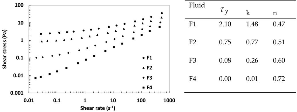
Figure 4 (left) Rheogram of Carbopol solutions used as carrier fluid in channel trials. (right) Herschel Bulkley model parameters for test fluids
