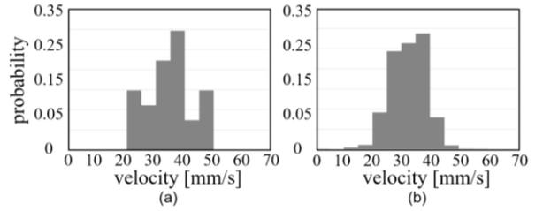
Figure 5: Probability density distribution of the sedimentation velocity from (a) echo intensity method, and (b) PTV
